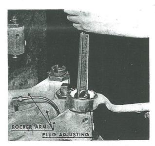
Fig. 82. Adjustment of Zero Lash Unit
