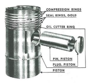
Fig. 103. Piston with Piston Pin Removed
