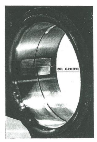
Fig. 119. Oil Grooves in Bearing Shells
